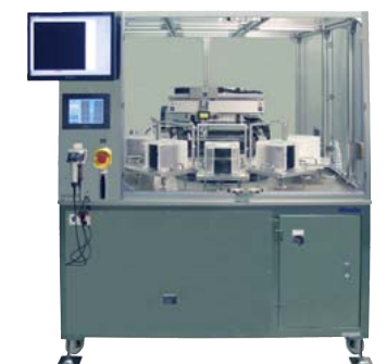
In-line inspection equipment with automatic wafer handler
